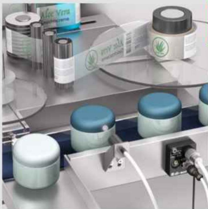
Color sensor FSB 10 M G1-B8 Fiber-optic cable WRB 120 P-SG M6x30-2.5 Attachment optics VO-M6/35-M6x30-2.5
